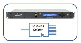
The *ViaLiteHD* Multizone Distribution Lossless Splitter allows for multiple receive points to be supplied by one transmitter with zero optical loss. It can be used with any *ViaLite* RF over fiber frequency band, but is typically used in any fan-out application in satcom or timing applications, such as GPS or 10 MHz reference. The lossless splitter utilizes the low loss 1550 nm wavelength or any of the ITU DWDM channels for longer distances.
