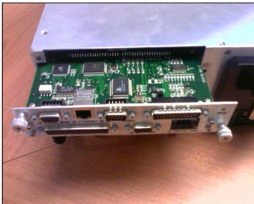
Removable rear panel monitor and control card
