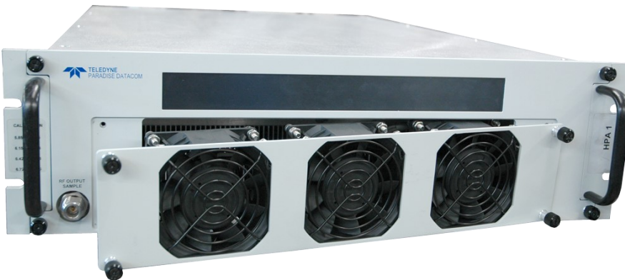
Removable front panel fan tray
