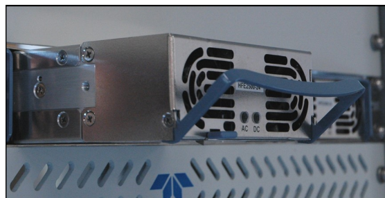
Power Supply Module in Chassis
