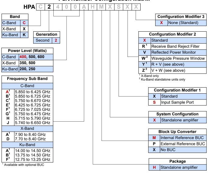
**Example** - A standalone 400W GaAs C-Band High Power Outdoor SSPA an optional input sample port and optional internal reference block up converter is part number: HPAC2400AHMXSXX.
