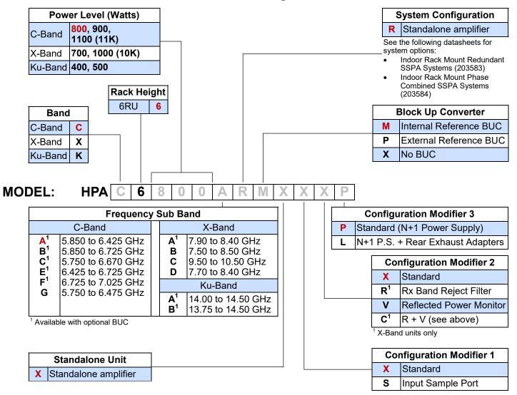
**Example** - A standalone 800W GaAs C-Band 6RU Rack Mount SSPA with standard N+1 external power supply and an optional internal reference block up converter is part number: **HPAC6800ARMXXXP**.
