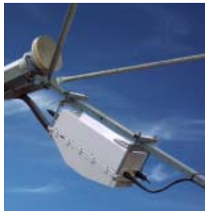
C-Band Medium power Block Up Converter
