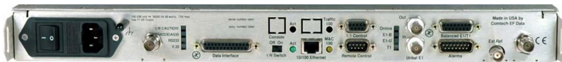
CDM-570 Satellite Modem Back Panel
